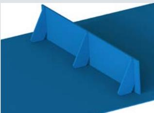
Gussets can be welded to the reverse of the cleat to provide support. Gussets should be positioned according to the width of the cleat, the load supported and its distribution on the cleat.
